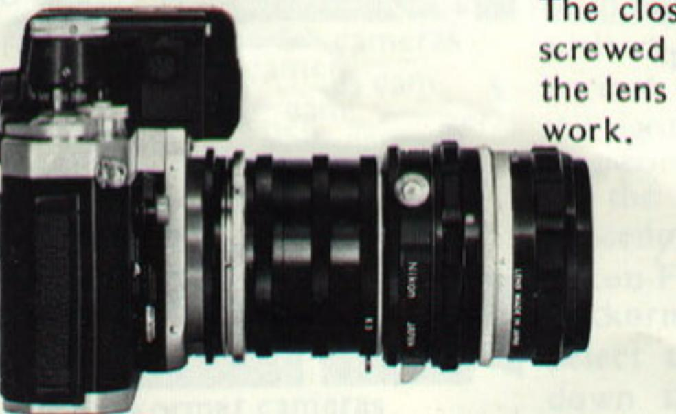
For greater reproduction ratios, the K Ring set can be combined with other closeup accessories such as bellows focusing attachments, E2 Ring etc. For example, the E2 Ring not only gives an extra 14mm lens extension but also permits semi-automatic diaphragm control with Nikkor Auto lenses. The close-up attachment lenses can also be screwed onto the front of the lens. However, the lens should be stopped down for critical work.
