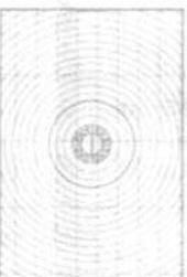
**Type K:** Combination of Type A and J screens. Matte/Fresnel field with 3mm split-image rangefinder spot surrounded by 1mm-wide microprism doughnut. Rapid and accurate focusing for subjects with both straight lines and ill-defined contours. Suitable for general photography.
