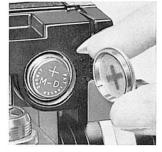
To exchange the mercury (Hg) battery, open the battery chamber by unscrewing the lid. Insert the battery into the chamber as its plus (+) side faced outward, so that this (+) side comes into contact with the inner side of the lid marked plus (+).
